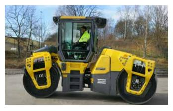
have very good control of the front drum edges and can follow a curb or other obstacles with a high degree of accuracy.
